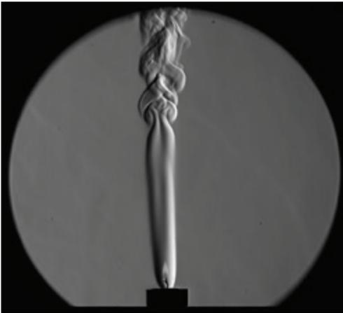
**Figure 2:** Thermal plume.
