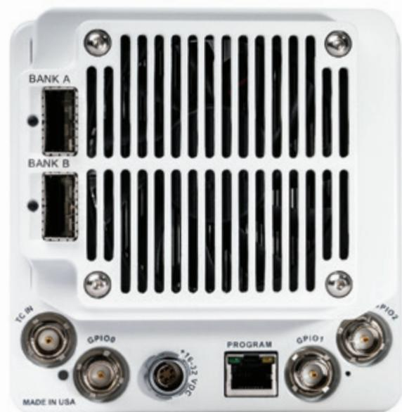
*The Phantom S991 provides the same throughput as its predecessor, the Phantom S990, but it uses only two QSFP+ transceiver modules and fiber cables.*
