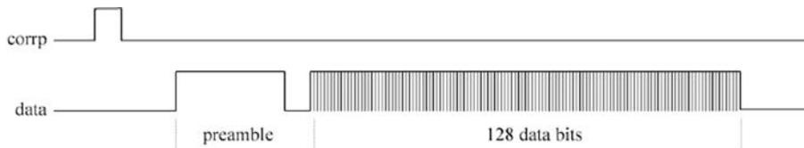
After the preamble is detected, the 128 data bits following are shifted into a shift register. On the rising edge of the next correlation pulse, the data from the shift register is combined with the current time, and sent to the recording system. After that, the shift register is cleared and made ready for shifting in more data.
