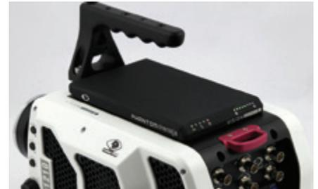
CineMag II installed on a Phantom v1210 camera
