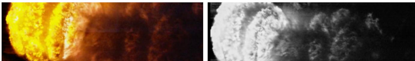
*Filming high-speed combustion events like this detonating cord and TNT in color (233,333 fps at 1280 x 256) versus monochrome (308,823 fps at 640 x 384) can provide additional details about the event despite the lower frame rates.*
