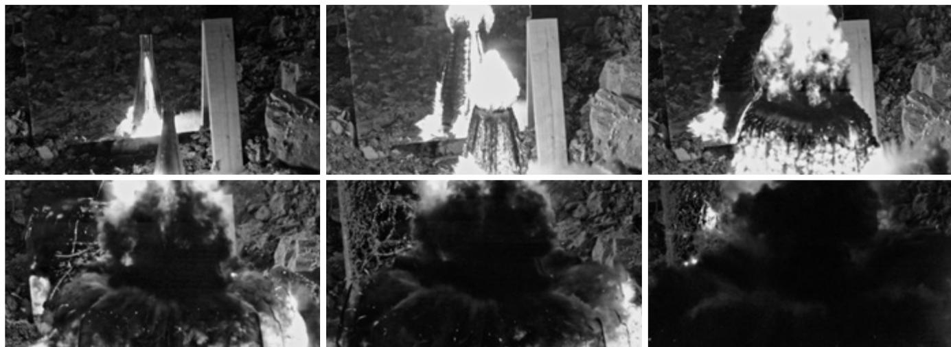
*Exploding shape charges filmed using a mirror. 456,521 fps at 640 x 256.*
