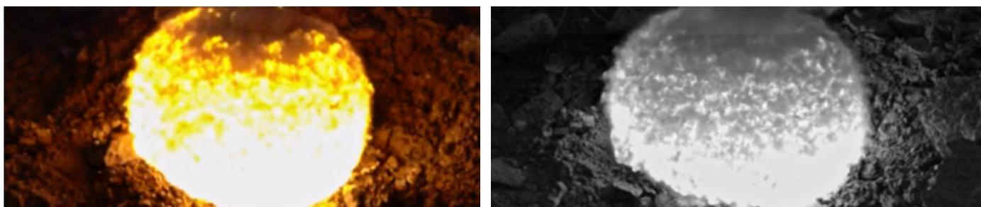
*Exploding dynamite in color (233,333 fps at 512 x 256) versus monochrome (617,647 fps at 512 x 192).*
