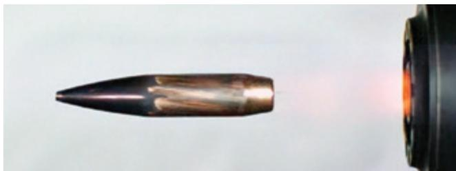
*High-speed footage of a ballistics test featuring a 338 Lapua Mag. 308,823 fps at 1024 x 192.*
