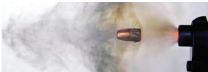
*High-speed footage of a ballistics test featuring a 9mm round. 187,500 fps at 1024 x 320.*
