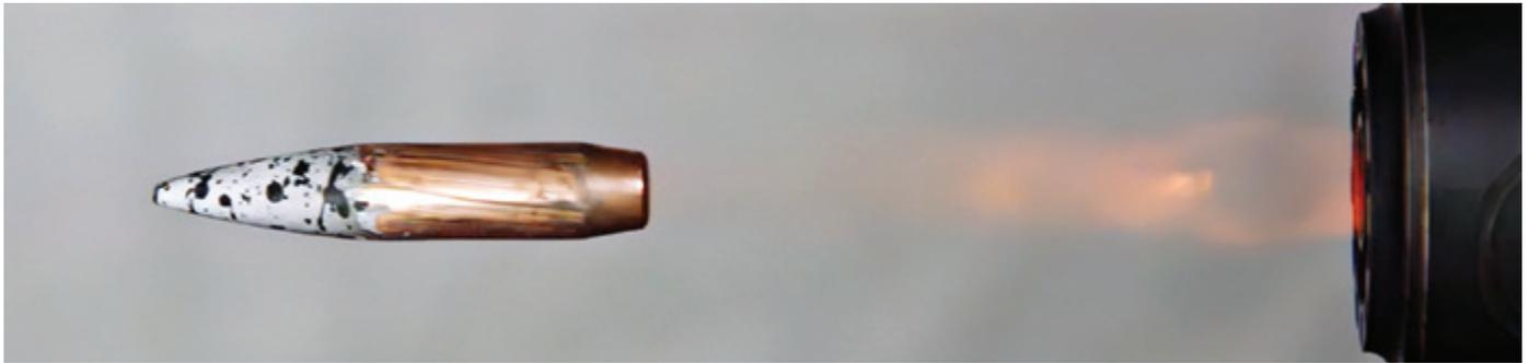
*McIntyre applied a speckled pattern to the 338 Lapua Mag cartridge as part of DIC analysis. 308,823 fps at 1024 x 192.*
