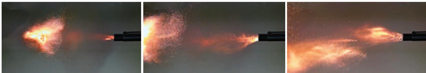
*High-speed footage of dragon's breath, an incendiary-effect round for 12-gauge shotguns. 86,065 fps at 1024 x 704.*
