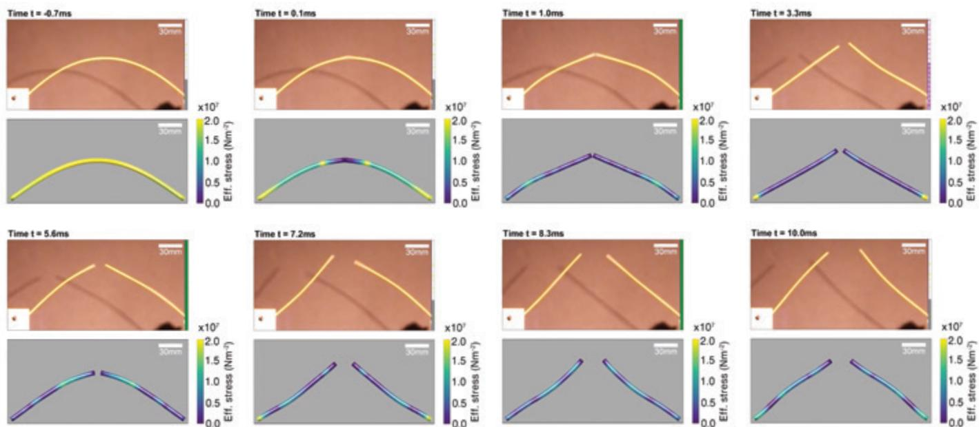
Binary fracture of spaghetti is observed in both trials and simulations at high twist angles ( $330^\circ$ ). Frame rate = 1,972 fps.
