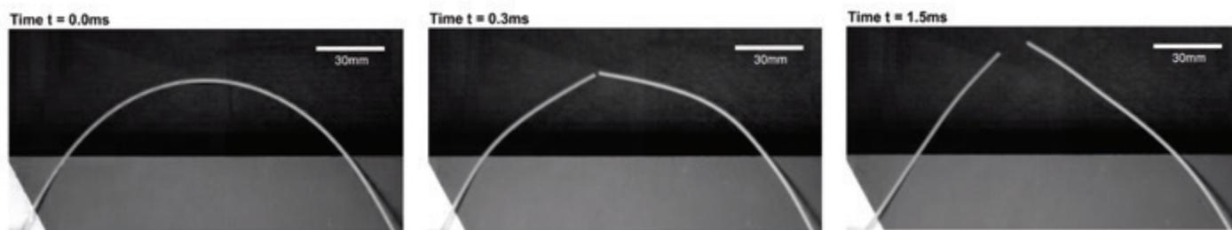
*Binary fracture of spaghetti may be induced at low quench speeds (2 mm/s). Frame rate = 75,000 fps.*
