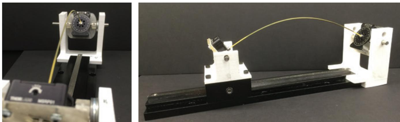
For their experiments, the MIT team constructed a custom device to controllably break hundreds of 24-cm spaghetti sticks with controlled twisting forces and nonadiabatic quenching.
