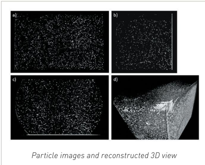
the v1610 offers 28-micron pixels that allow for superior sensitivity when shooting in low light, which was an issue during Brücker’s experiment. “We couldn’t use a traditional lighting setup for this type of application because it would have hampered our results. The only lighting we had during testing was the light from the laser that was diffused over the sheet. But that proved to be enough, because the v1610 performed flawlessly,” he said.
