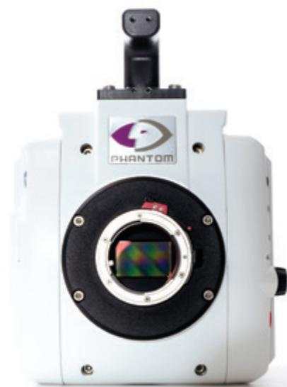
*For their DIC experiment, researchers used two high-speed Phantom v1612 cameras, which can shoot up to 16,000 fps at full resolution.*
