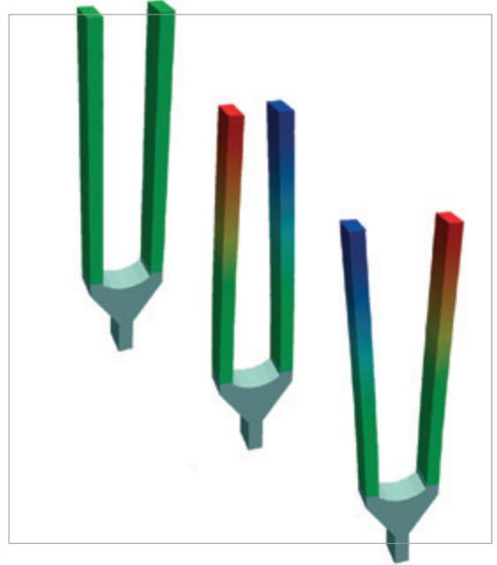
*The team also used the DIC data to generate Operational Deflection Shapes (ODS) of the tuning fork's vibration pattern.*
