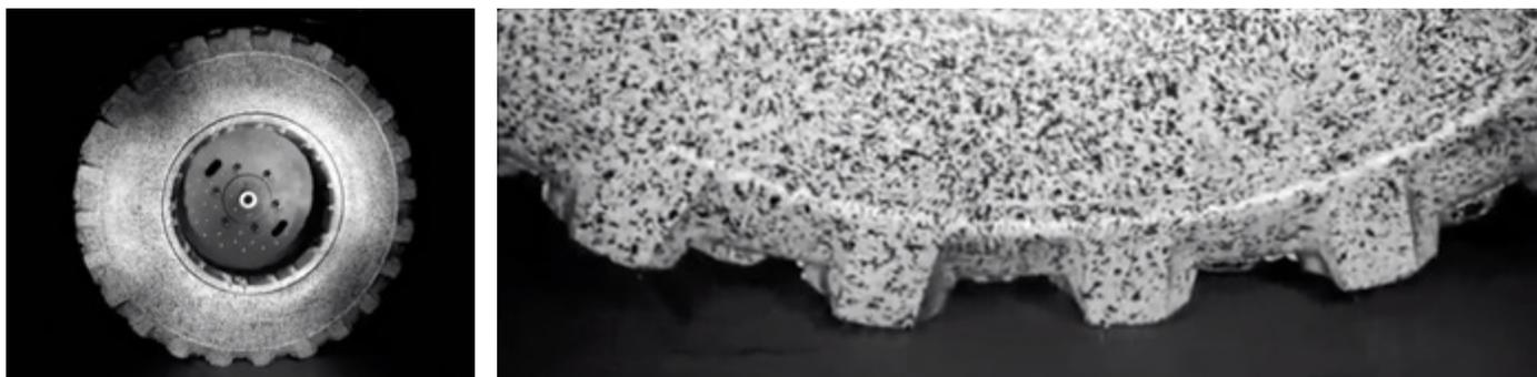
*DIC utilizes a speckle pattern that is painted onto the object’s surface to provide focus points for the cameras during high-speed filming.*
