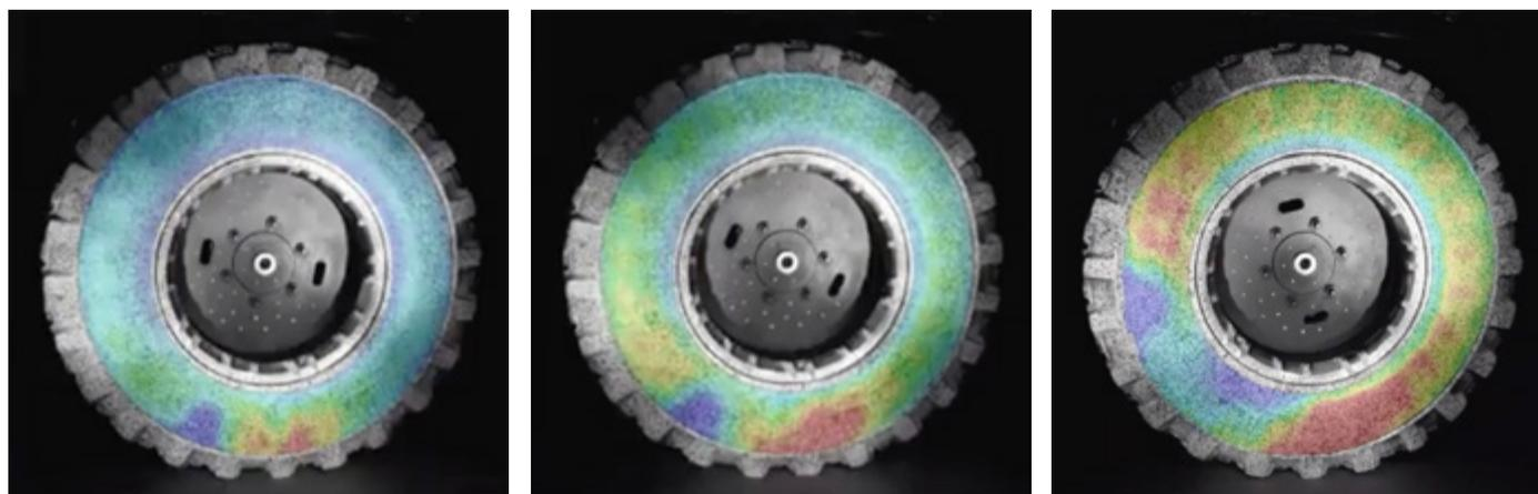
*Phantom v2640 cameras recorded the tire accelerating at 4,800 fps at 2,048 x 1,952 resolution. To evaluate surface displacement and strain, the team ran the footage through GOM Correlate, which expressed micro-level surface deformations as colored deviations.*
