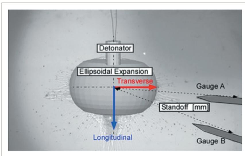
Figure 5: Approximated blast wave generated
