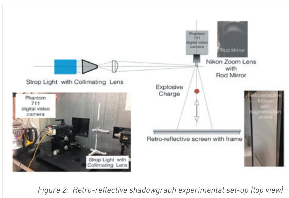
Figure 2: Retro-reflective shadowgraph experimental set-up (top view)
