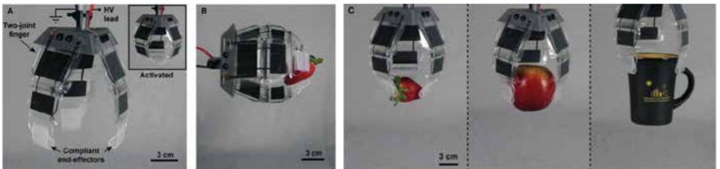
Several joints can be arranged one behind the other like a finger - and combining multiples of them can form a hand. This can be used to lift a strawberry, an apple or a coffee cup.
