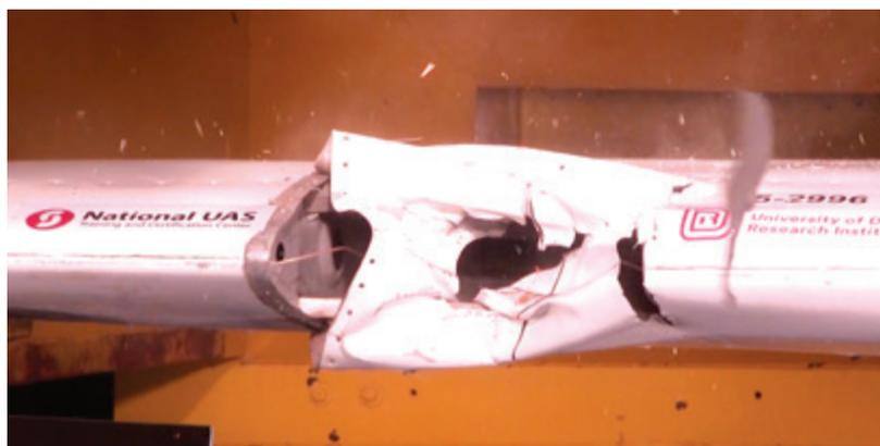
*The ballistics team fired a drone at the aircraft wing to simulate a midair collision at 238 mph.*
