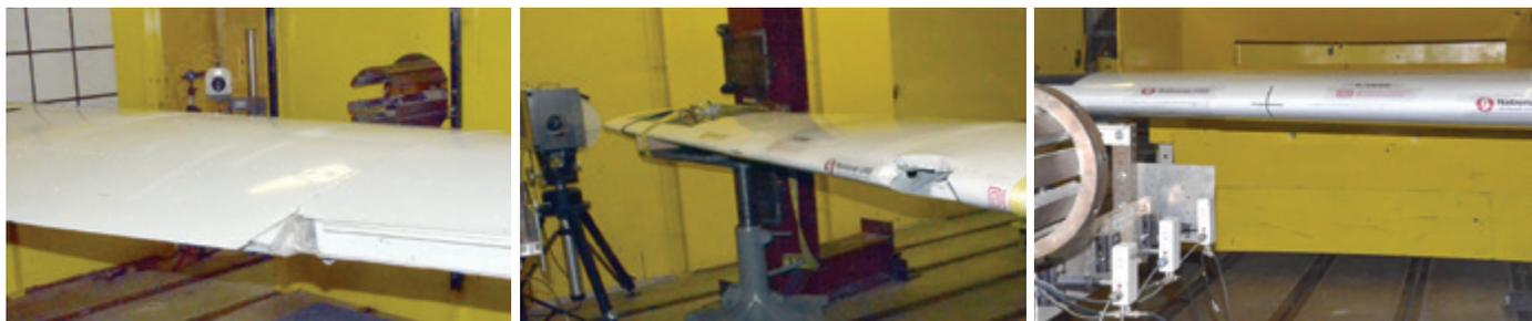
*Capturing the simulated collisions were three Phantom v2012 high-speed cameras positioned at the top and sides of the wing.*
