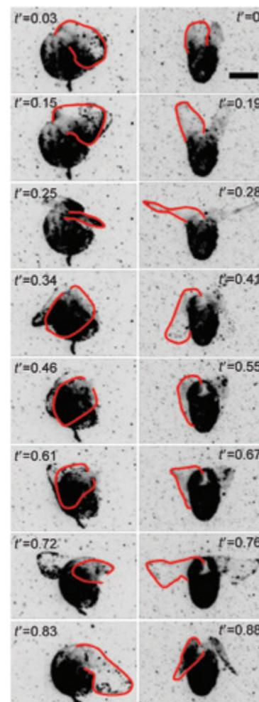
*Sequence of inverted-color PIV images for two sea butterflies, illustrating the stroke cycle. One wing in each image is outlined in red.*
