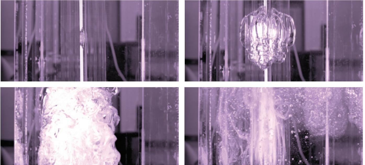
*The researchers recorded a simulated fuel element break using two Phantom VEO 340L cameras at 800 fps. Each point of analysis is 5 ms apart.*
